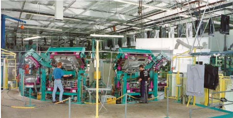
Rotating die-casting equipment of Krauss-Maffei Kunststofftechnik (Munich); in operation at Johnson Controls Interiors (Lüneburg)
